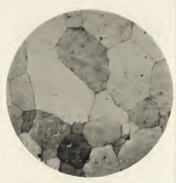
Fig. 16. Type of class 1. Steels containing from 0 to 1.6 per cent P. Magnified 50 diameters.
